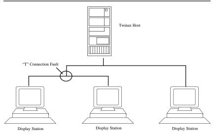
Other problems that the Twinax Monitor Mode can help diagnose are defective twinax devices, and defect pigtails. These sorts of problems would be indicative of the Twinax Monitor Mode reporting parity errors for all of the active addresses of a particular twinax device, while the rest of the twinax devices do not report parity errors for their active addresses.
